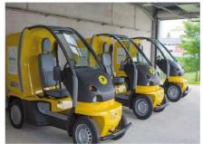
Fig. 1: Mobypost vehicles – First fleet of FCV in France (FC powertrain integrated @ FCLAB / UTBM)
