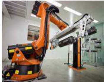
Figure 1: CEA (Monts, F-37260) Robot assisted filament winding unit.
